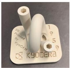
CAM printing technology can be used to produce parts in complex shapes.
